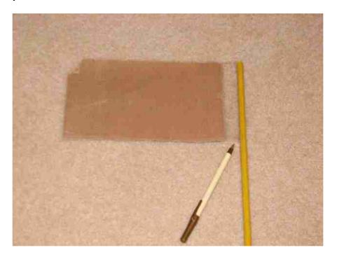
Where the pen is pointing is clear box tape wrapped around the rod and overlapping the sandpaper on both sides for an inch or so. Now wrap the sandpaper tightly around the rod with the grit facing out.
