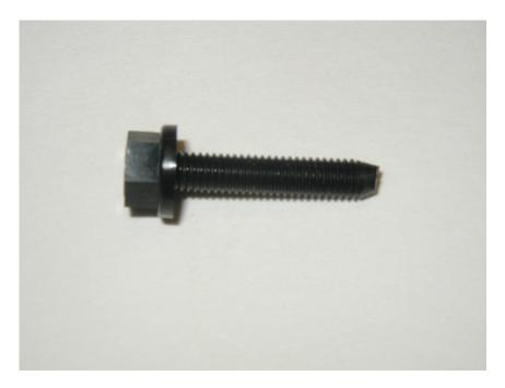
Note the bevel on the leading end of the bolt compared to what we started with. Now you have a nylon bolt that is the right length for the job and actually starts a lot easier than before. Give it a try; you might be surprised how well this works.
